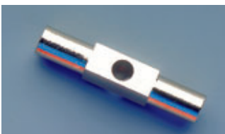
SFC/CO Cat. No. FC102 Ø 6,3 x 32 mm - in brass for terminal block types: FPC.10 - SFC.10 - SFR.6 - with the option of inserting an SDD/2 test plug
