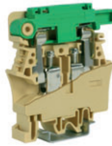
The terminal block is equipped with a lever suited to house a \varnothing 6.3 x 32 mm - 500 V fuse and a non-polarised LED microcircuit. The interruption of the fuse determines the ignition of the LED. The terminal block can be supplied with the CIL circuit already mounted for the insertion of a non polarised LED circuit.
